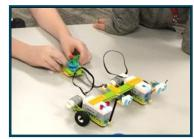
Fourth and fifth grade students used micro:bits to create "robots". They built a Rover using Lego pieces, 2 servo motors, a micro:bit and a Bit Board. After building the Rover, they experimented with the code to make it operate differently.
